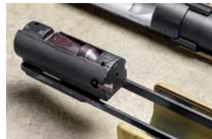
The bolt rides on twin action bars and a locking block that will look familiar to owners of other pump-action shotguns.
