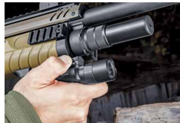
The rail at 6 o'clock is well suited for attaching a small light or laser. A handstop is integrated behind the bottom rail.
